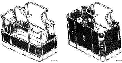
Figure 32. Platform Mesh to Mid Rail
