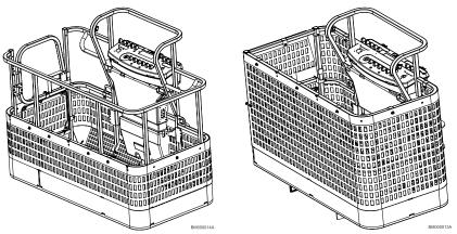
Figure 28. Fabric Mesh to Mid Rail
