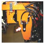
Figure 48. Platform Filter — S Models
