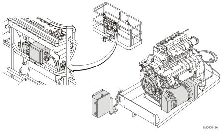
Figure 37. SkyPower and Generator Systems
