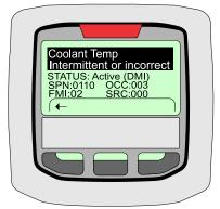
Figure 8. Engine Diagnostic Screen
