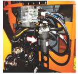
Figure 49. Platform Filter — SJ Models
